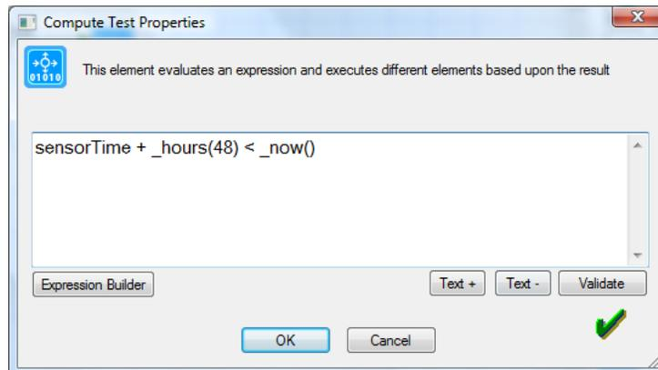
In both these elements the Validate button is used to check that the expression you have entered is correct – it matches the syntax that HCA expects.
