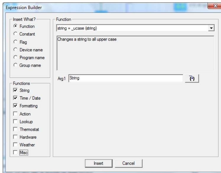
The upper left box specifies what sort of item you are inserting. The most common case is one of the HCA build-in functions.
