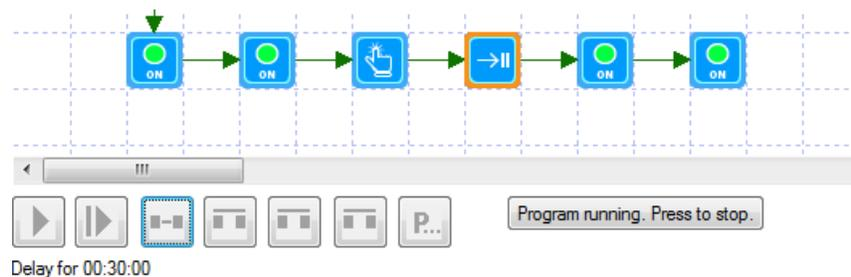
Note that the buttons to control the debugger have been disabled and an additional button has appeared. This button when pressed aborts the execution of the current element – in this example a *Delay* element. Once you stopped execution of the current element you can move to the next element by using the *Skip* button or by changing the current element as described above.
