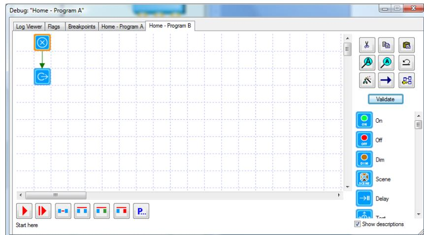
Note that the current element for program B is the *Begin-Here* element. If you switch back to the *Program A* tab, the current element is still at the *Start-Program* element since it has not yet completed.
