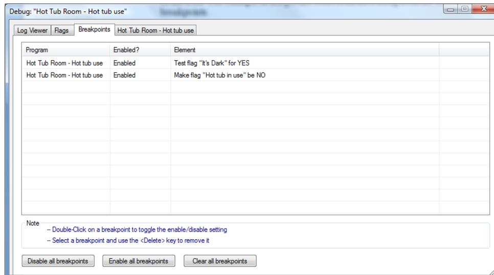
In addition to being set on an element, a breakpoint can be enabled or disabled. When you first add a breakpoint it is automatically enabled. If you no longer want execution to stop at that element you can disable or remove the breakpoint.
