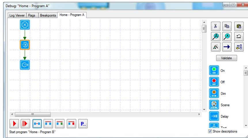
Press the *Step* button and the current element becomes the *Start-Program* element. Press the *Step* button again and the *Start-Program* element executes and a tab for program B appears.
