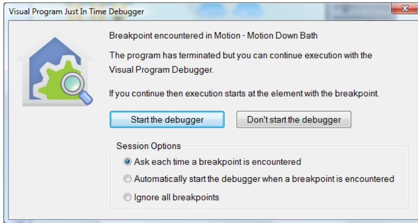
If you press the *Start the debugger* button then the debugger opens and the current element – the one with the breakpoint that has not yet been executed – is designated with the orange border showing it is the current element.
