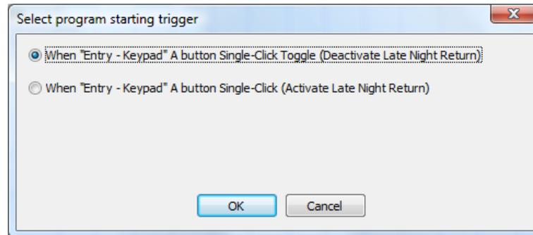
This program has two triggers. If there were other triggers then additional options or a dropdown would be shown so you can select the trigger to use.
