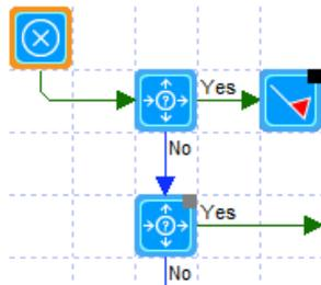
The *No* path from the test element has a disabled breakpoint. The *Yes* path element has an enabled breakpoint.
