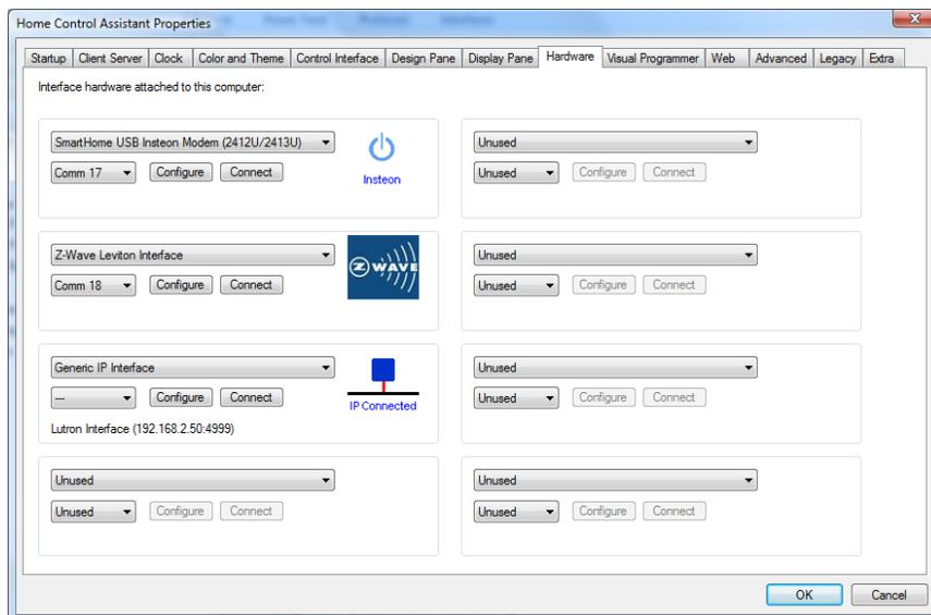
HCA supports from one to eight automation interfaces attached to your computer. Each must be attached to its own serial or USB port, or accessed via a network connection.
