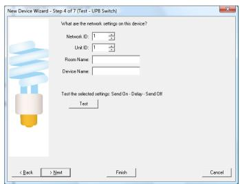
In this dialog you must enter the network id and unit id as well as the room and device names for the new unit. Once the device is added this way you can control it as a normal UPB device.
