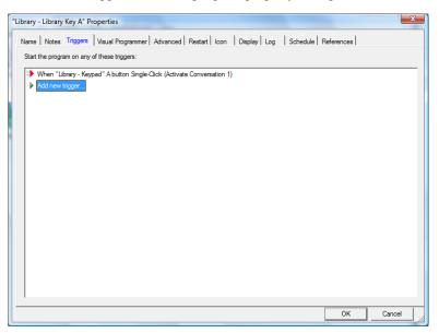
There are two different types of UPB triggers you can create. UPB Action and UPB Powerline Message triggers.
