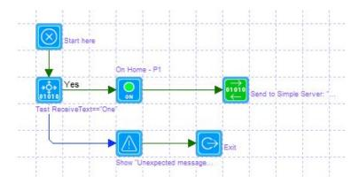
The program checks to see if the reception text is "one" and if so it starts the "P1" program and then replies back to the client – in this case the web page that opened the web socket. The Port-IO element is used for that message transmission and is the same as used by the generic serial interface and the generic IP interface.
