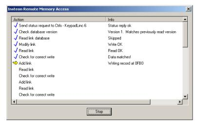
Actions that complete without error are checked off when done. The current action is shown with the yellow arrow, and operations that fail show with a red X.
