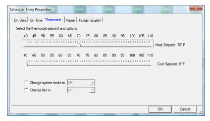
Depending upon the model thermostat in use the options may be different. To change the setpoint drag the thumb of the slider to the desired setpoint. To change the other options enable the option with the checkbox and select the option value from the dropdown.
