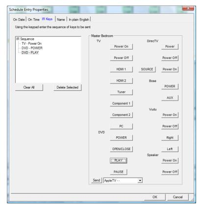
The contents of the dialog depend on the keypad used by the IR device. In this case a custom keypad for this television was created with the keypad builder. The keycodes sent when this schedule entry happens are shown in the box at the left side of the dialog
