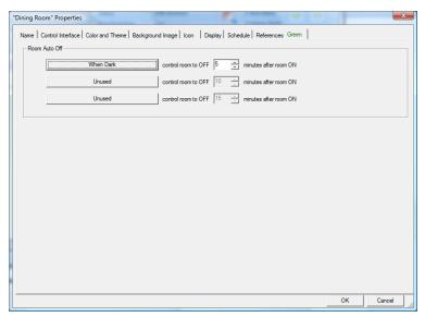
In the same way that a device auto-off is configured, you can have up to three different auto-off specifications. In the above example, 5 minutes after the room is tuned on – when it's dark – the room goes off. This means that any devices in the room configured to respond when the room goes off, are sent a command to go off.
