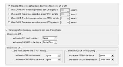
The action of turning on either light causes the room to go ON. Since the room was OFF and an ON was received then auto-off timer is started. Controlling the other light causes the timer to be canceled.
