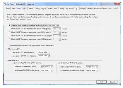
There are a lot of options on this dialog and they will all be covered in the chapter. For now only the first checkbox is important. If that checkbox is ticked then the device participates in determining the room state as described above.
